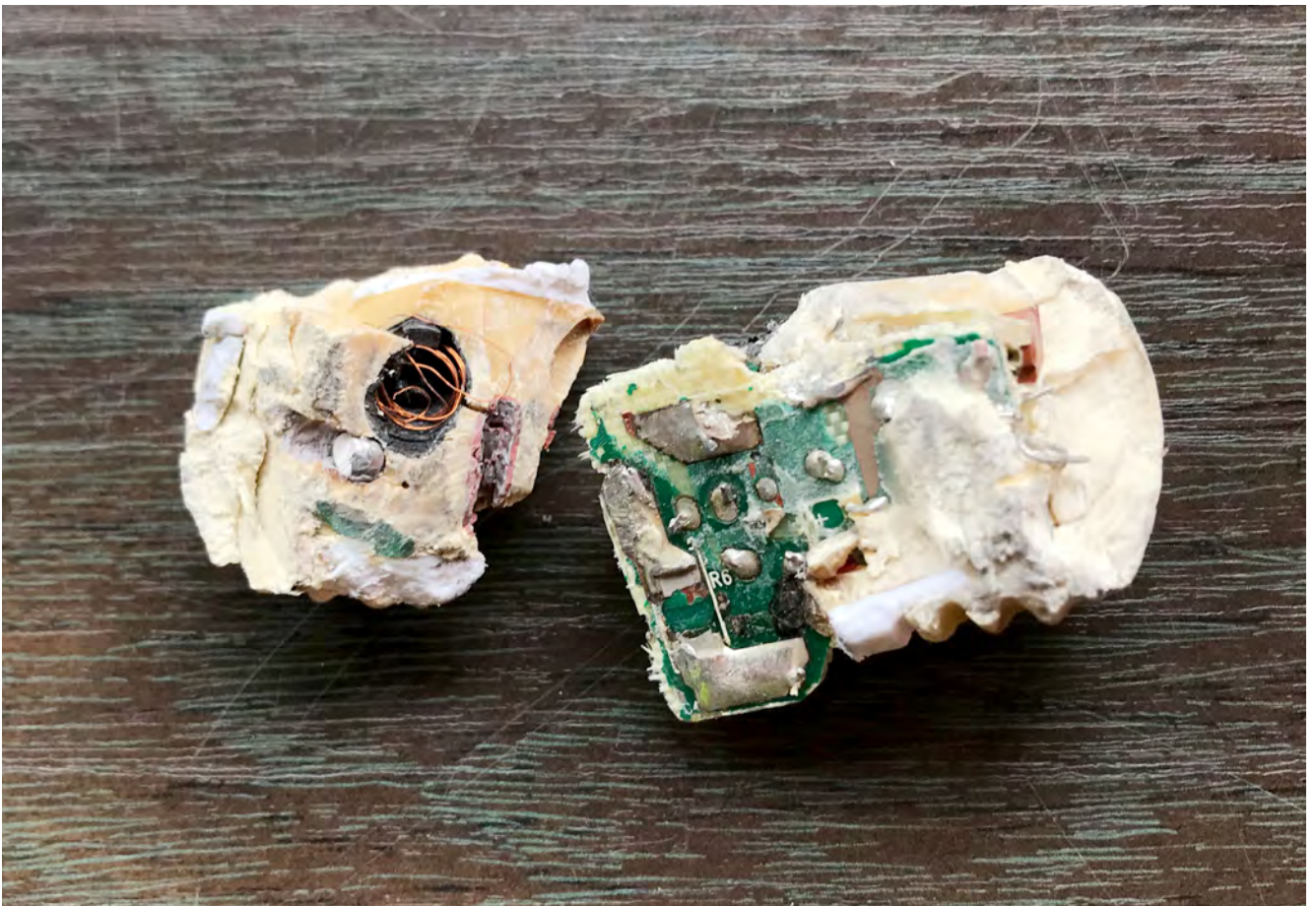
Photo 2: The valuable printed circuit boards are embedded in certain LEDs.
