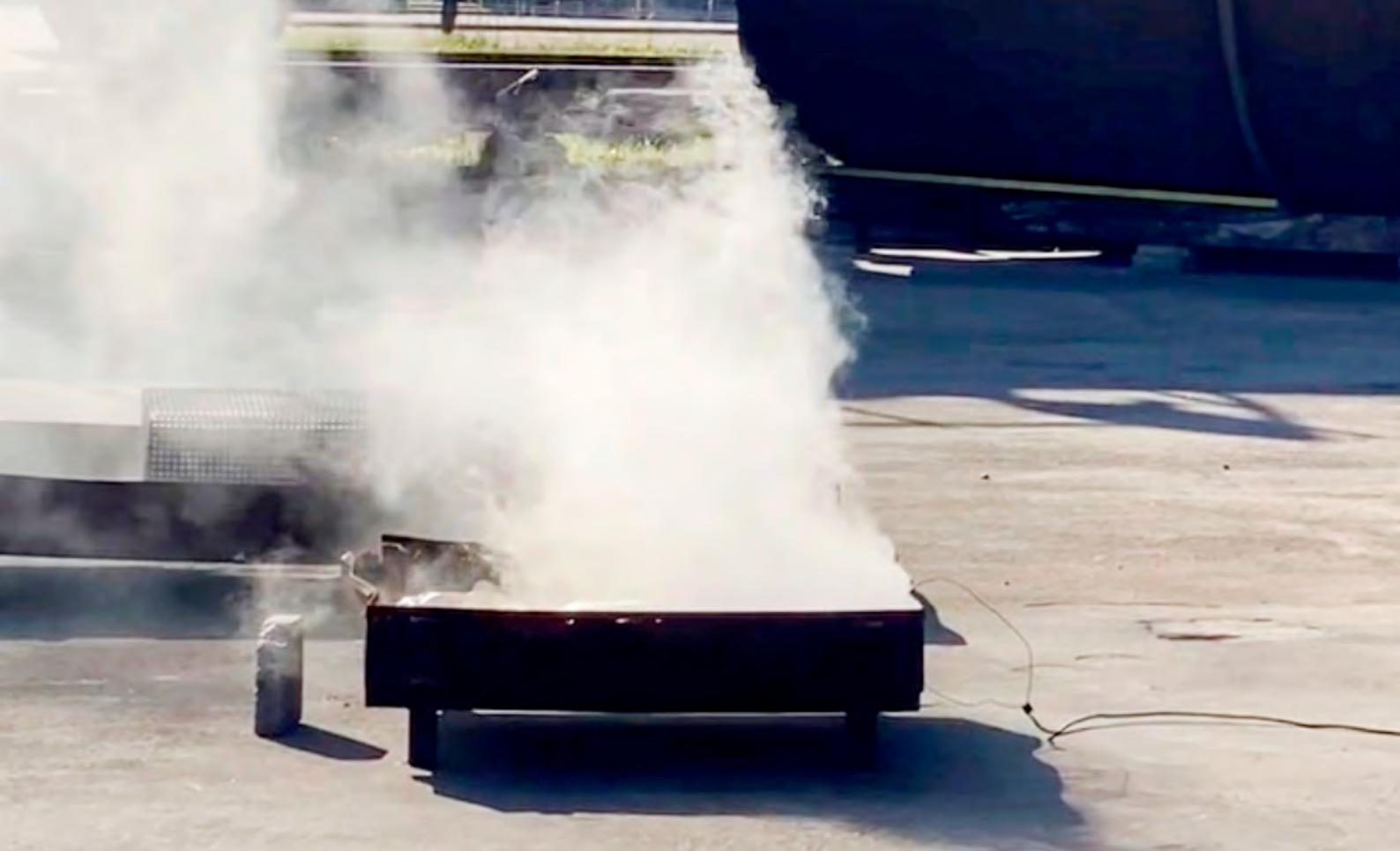
Photo 2: Phase 1 – The “thermal runaway” (chain reaction in the battery) due to the short circuit of individual cells.
